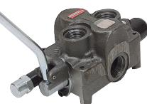
• Brand new, BRAND HYDRAULICS high flow directional control valve. Cast iron body with Buna-N O-rings. High lift, ball spring relief valve. Handle included.
